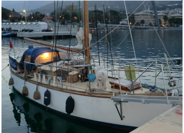
Passerelle rigged showing supporting bracket
